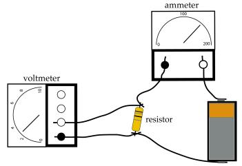
2. Add a second battery in series with the first as shown. Write down the new voltmeter and ammeter readings in table 1.
