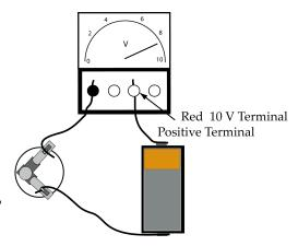
2. Draw a circuit diagram for the circuit below. How is the voltmeter connected now?
