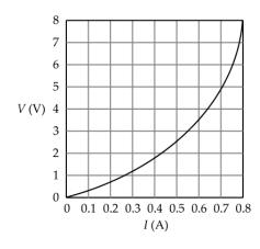
Use the graphs to calculate the resistance of the resistor when the current through it is 300 mA, and when it is 600 mA. Do the same for the bulb. Write your results in the table below.
