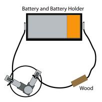
The box shown at right contains a material which is connected to the two wires. Describe an experiment which allows you to tell whether the material is a conductor or an insulator. Draw a diagram, and state how you would decide.
