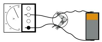
Set up the circuit. Does the bulb light?
