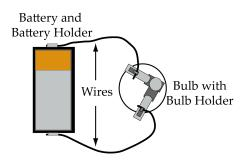
Set up the circuit. Try and remember how bright the bulb is.
