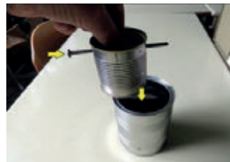
Figure 5.3 A: Assembling the calorimetre.
