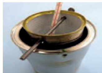
Figure 5.4: Measuring water temperature in the calorimetre.
