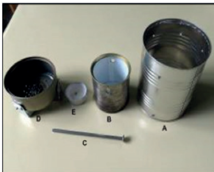
Figure 5.2: Materials to make the calorimeter.
